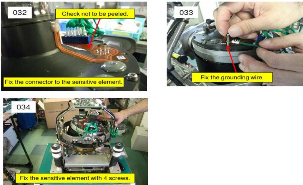
Figure 11: Mounting of Sensitive Element part 2
