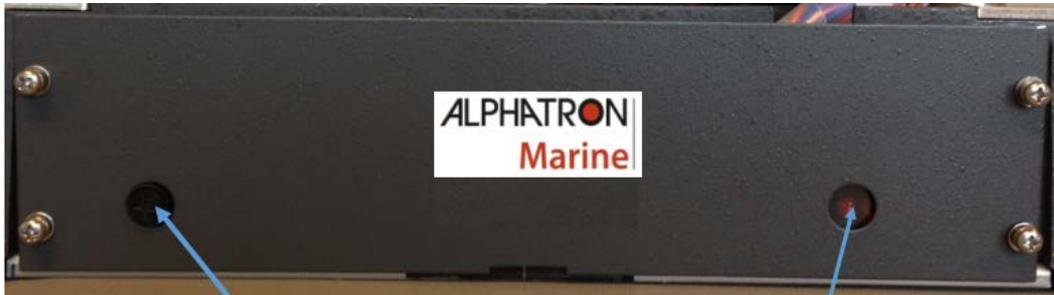
Gyro compass Inverter unit: Fuse 12A ( 6x32 )
