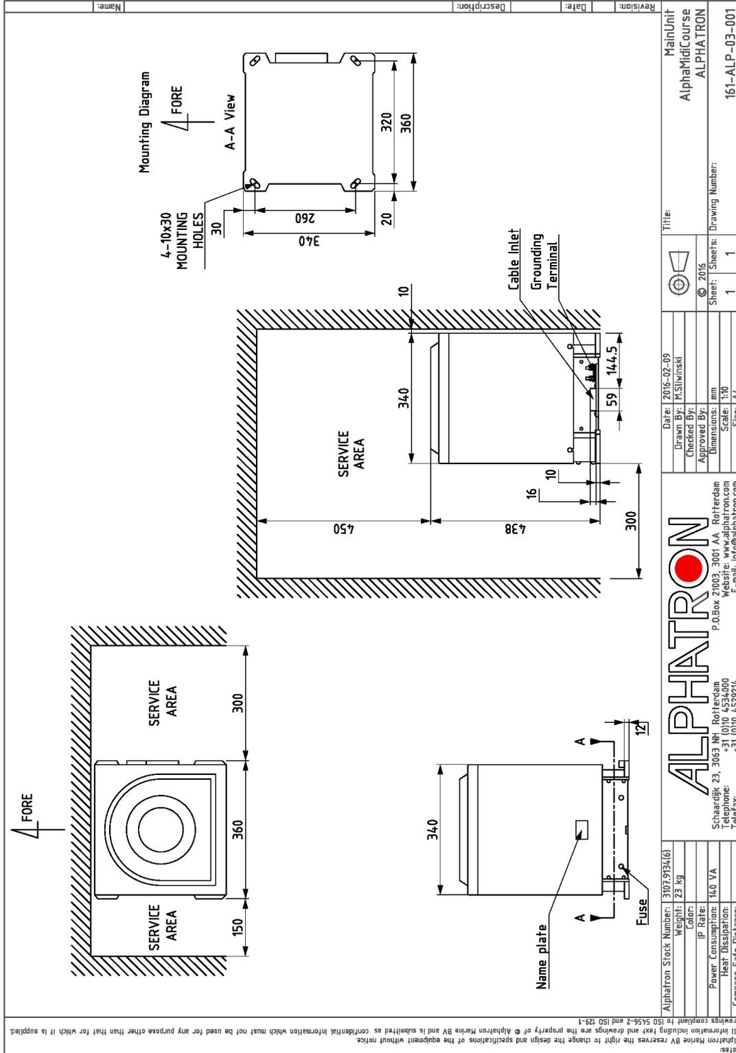
Figure 48: Installation Drawing
