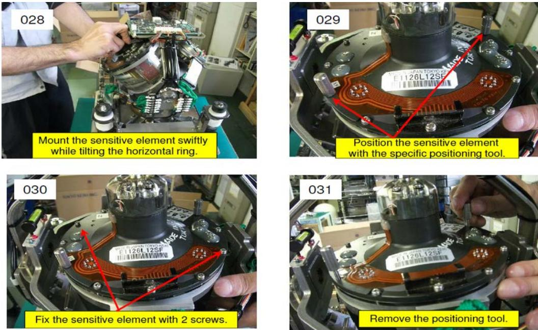
Figure 10: Mounting of Sensitive Element part 1
