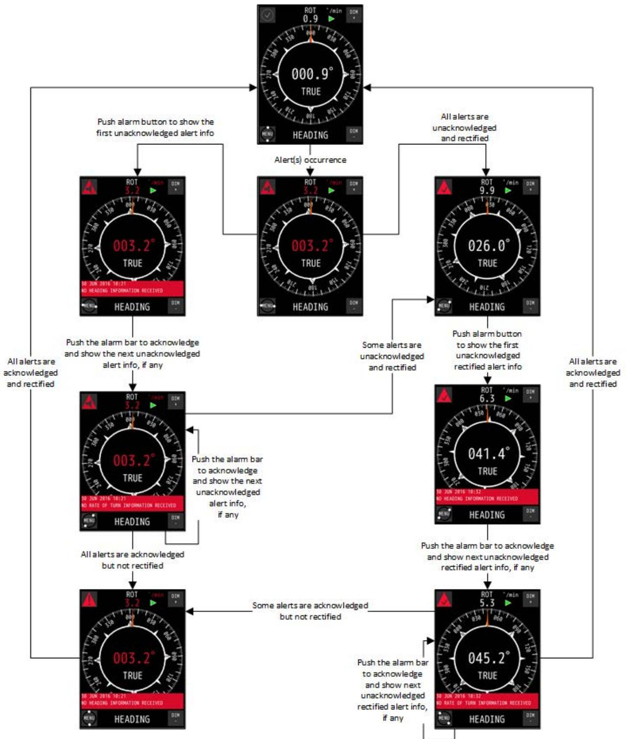
Figure 21: Alert Handling in Main Screen (example)
