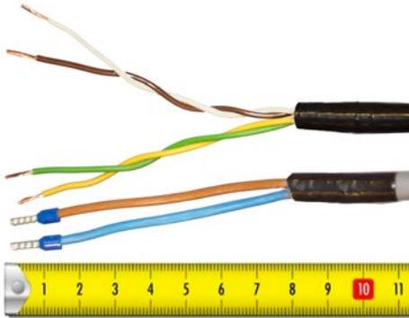
**Figure 9: Cable Preparation Receiving Cable Sides**
