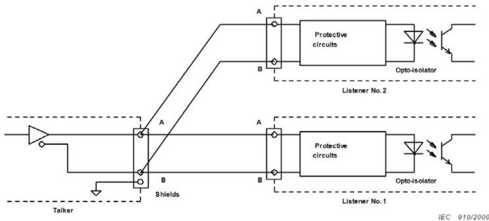
**Figure 11: IEC 61162-1 Circuits**
