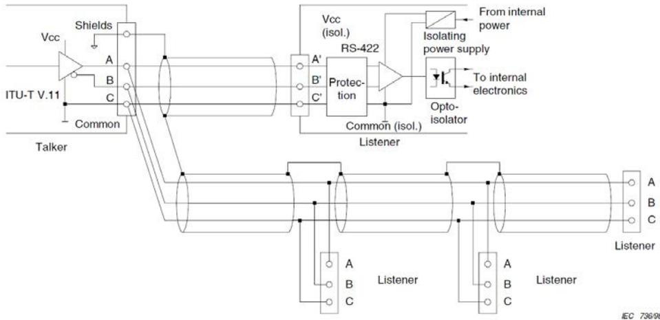
**Figure 12: IEC 61162-2 Circuits**
