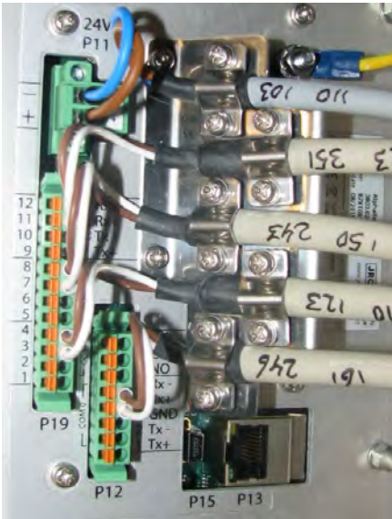
Figure 10: Serial pin connections
