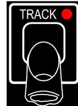
The Track key corner red LED will also be illuminated and the operating mode shown on the display will be "**AUTO TRACK STEERING**".
