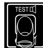
The audible alarm function can also be permanently turned **OFF** (muted) by continuous 5 second press of the "**TEST/OFF**" keypad and is confirmed by the Alarm icon at the bottom left corner of the Control Unit display.
