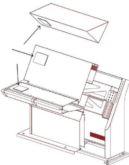
**Figure 1: Flush mounting**
