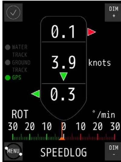
Figure 18: Main Screen AlphaSpeedLog Aft
