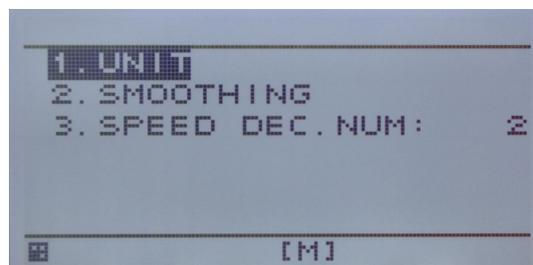
The speed unit can be switched kn and m / s and is explained in 5.2.1.
