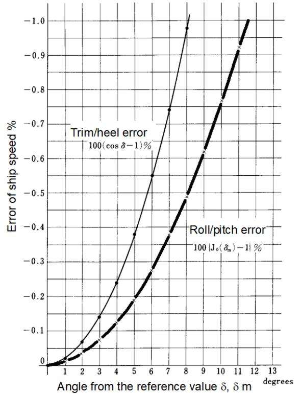
Figure 4 Errors by vertical slopes in dual beams
