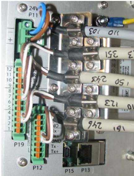
Figure 12: Serial pin connections
